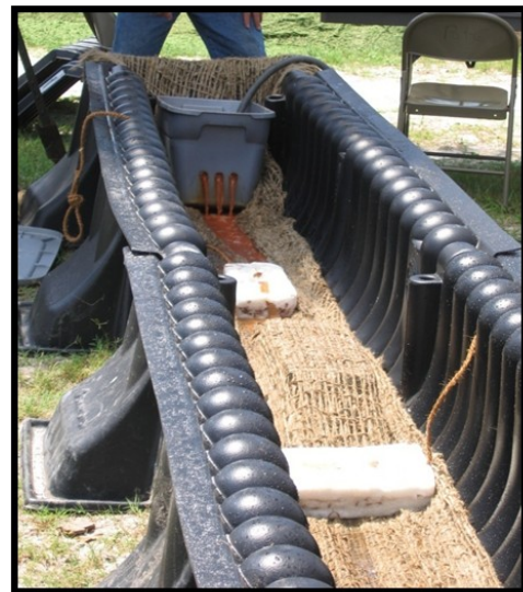
(As the water flows over and around the floc logs, the polymers mix with the water and form particulates that adhere to the jute matting.)
